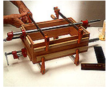
6 -- The waterproof glue sets quickly, so six clamps and cauls must be ready. Position the clamps and cauls as shown.
