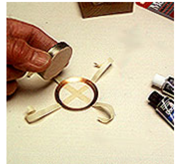
18 -- Seal the flange with epoxy and let it set. Then, tape the flange to the humidifier and fasten it with epoxy.
