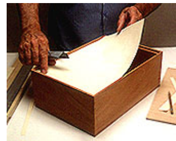
7 -- Make a cardboard template of the top panel. Test it in the rabbet-it should fit in the space snugly.
