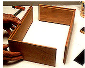
5 -- Make two L-shaped subassemblies, each comprised of a side and an end. Press the subassemblies together.
