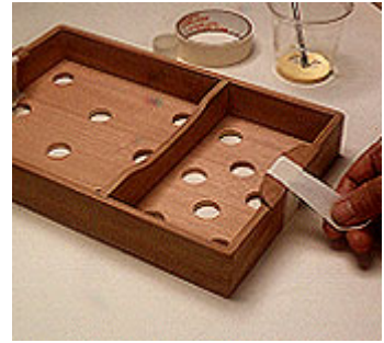
15 -- After the tray is sanded, apply glue on the handles and hold them in place with masking tape until the glue sets.
