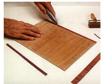
9 -- Use a sharp knife to trim off the excess veneer. Cut from both ends toward the panel's center to prevent tearout.
