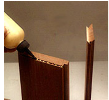
4 -- Apply glue sparingly and evenly in the spline slots. Use a hair-colorant squeeze bottle with a fine nozzle.
