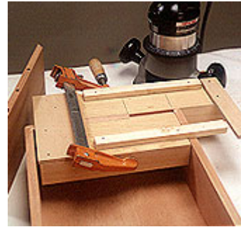
13 -- Cut the mortise for the lid support using a router and jig. Try the cut on a scrap piece first.
